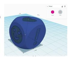
By hiding, or removing, the cube. We can now see the symbols on their own. They are made solid again, grouped, and exported as a separate object to form the symbol (or positive) portion of the die.
