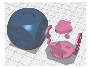
Finally, the two objects are merged. As they have been designed to fit together, Cura is able to logically merge them into the final object we want to print.
