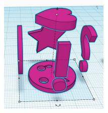
In Cura, we import these two object files. The objects are selected individually. The cube portion is selected for Extruder 1, which will use the blue filament. The symbols are designated for Extruder 2, which will use magenta filament.
